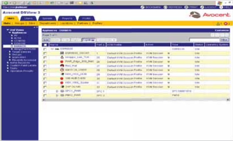
Figure 4. Each blade server attached to the HP adapter and the DSR KVM switch appears as a target device in the main DSView 3 software interface.
