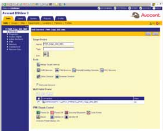
Figure 6. The target device, PWR_Edge_800_BMC, is accessible through a KVM, IPMI, SoL, or RDP/VNC connection.
