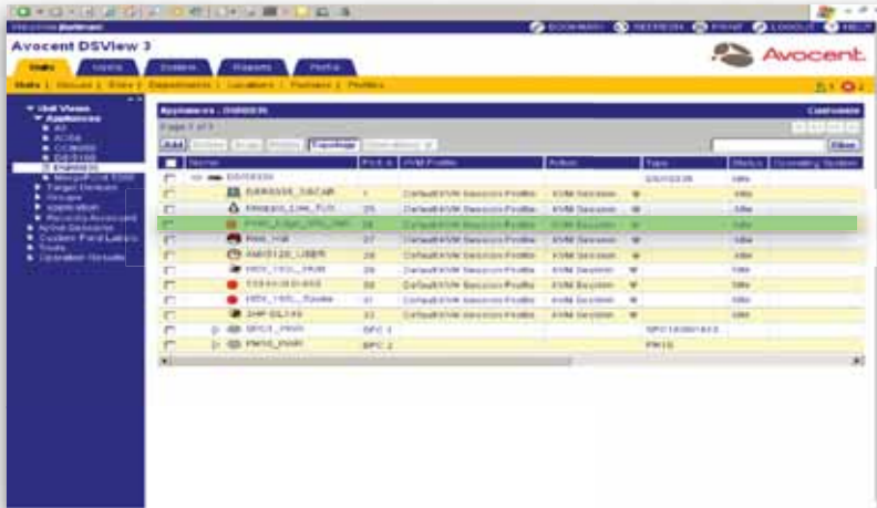
Figure 5. Each blade server does not appear as a target device in the DSView 3 software interface.
